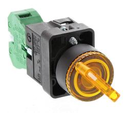
AutomationDirect selector switch, 22mm, 2-position, maintained, incandescent illuminated, (1) N.O. contact(s), plastic base, plastic bezel, Operator: yellow, knob, 30mm, round, plastic, 24 VAC/VDC, full voltage.
