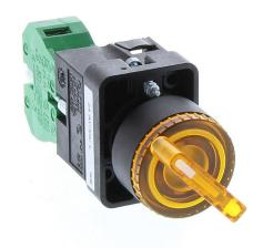
AutomationDirect selector switch, 22mm, 2-position, maintained, LED illuminated, (1) N.O. contact(s), plastic base, plastic bezel, Operator: yellow, knob, 30mm, round, plastic, 24 VAC/VDC, full voltage.
