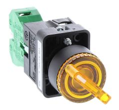
AutomationDirect selector switch, 22mm, 2-position, maintained, LED illuminated, (1) N.O. contact(s), plastic base, plastic bezel, Operator: yellow, knob, 30mm, round, plastic, 120 VAC/VDC, full voltage.
