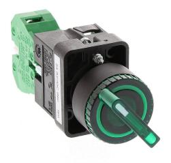
AutomationDirect selector switch, 22mm, 2-position, maintained, incandescent illuminated, (1) N.O. contact(s), plastic base, plastic bezel, Operator: green, knob, 30mm, round, plastic, 24 VAC/VDC, full voltage.
