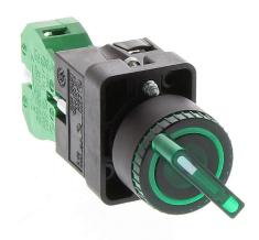
AutomationDirect selector switch, 22mm, 2-position, maintained, LED illuminated, (1) N.O. contact(s), plastic base, plastic bezel, Operator: green, knob, 30mm, round, plastic, 24 VAC/VDC, full voltage.
