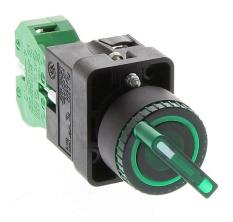
AutomationDirect selector switch, 22mm, 2-position, maintained, LED illuminated, (1) N.O. contact(s), plastic base, plastic bezel, Operator: green, knob, 30mm, round, plastic, 24 VAC/VDC, full voltage.
