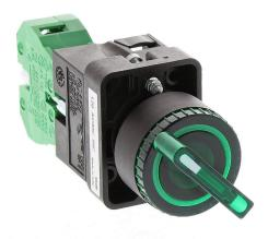
AutomationDirect selector switch, 22mm, 2-position, maintained, incandescent illuminated, (1) N.O. contact(s), plastic base, plastic bezel, Operator: green, knob, 30mm, round, plastic, 120 VAC/VDC, full voltage.
