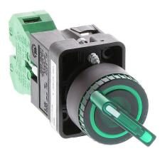
AutomationDirect selector switch, 22mm, 2-position, maintained, LED illuminated, (1) N.O. contact(s), plastic base, plastic bezel, Operator: green, knob, 30mm, round, plastic, 120 VAC/VDC, full voltage.
