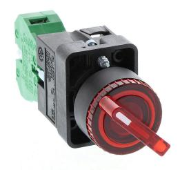
AutomationDirect selector switch, 22mm, 2-position, maintained, incandescent illuminated, (1) N.O. contact(s), plastic base, plastic bezel, Operator: red, knob, 30mm, round, plastic, 24 VAC/VDC, full voltage.
