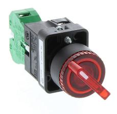
AutomationDirect selector switch, 22mm, 2-position, maintained, LED illuminated, (1) N.O. contact(s), plastic base, plastic bezel, Operator: red, knob, 30mm, round, plastic, 24 VAC/VDC, full voltage.
