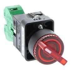
AutomationDirect selector switch, 22mm, 2-position, maintained, LED illuminated, (1) N.O. contact(s), plastic base, plastic bezel, Operator: red, knob, 30mm, round, plastic, 120 VAC/VDC, full voltage.
