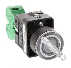
AutomationDirect selector switch, 22mm, 2-position, spring return from right, incandescent illuminated, (1) N.O. contact(s), plastic base, plastic bezel, Operator: clear, knob, 30mm, round, plastic, 24 VAC/VDC, full voltage.
