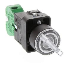
AutomationDirect selector switch, 22mm, 2-position, spring return from right, LED illuminated, (1) N.O. contact(s), plastic base, plastic bezel, Operator: clear, knob, 30mm, round, plastic, 24 VAC/VDC, full voltage.
