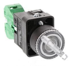
AutomationDirect selector switch, 22mm, 2-position, spring return from right, incandescent illuminated, (1) N.O. contact(s), plastic base, plastic bezel, Operator: clear, knob, 30mm, round, plastic, 120 VAC/VDC, full voltage.
