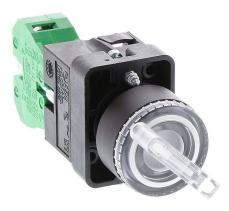
AutomationDirect selector switch, 22mm, 2-position, spring return from right, LED illuminated, (1) N.O. contact(s), plastic base, plastic bezel, Operator: clear, knob, 30mm, round, plastic, 120 VAC/VDC, full voltage.
