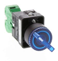
AutomationDirect selector switch, 22mm, 2-position, spring return from right, LED illuminated, (1) N.O. contact(s), plastic base, plastic bezel, Operator: blue, knob, 30mm, round, plastic, 24 VAC/VDC, full voltage.
