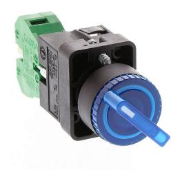
AutomationDirect selector switch, 22mm, 2-position, spring return from right, incandescent illuminated, (1) N.O. contact(s), plastic base, plastic bezel, Operator: blue, knob, 30mm, round, plastic, 120 VAC/VDC, full voltage.
