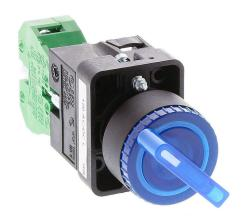
AutomationDirect selector switch, 22mm, 2-position, spring return from right, LED illuminated, (1) N.O. contact(s), plastic base, plastic bezel, Operator: blue, knob, 30mm, round, plastic, 120 VAC/VDC, full voltage.
