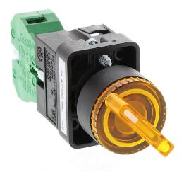
AutomationDirect selector switch, 22mm, 2-position, spring return from right, incandescent illuminated, (1) N.O. contact(s), plastic base, plastic bezel, Operator: yellow, knob, 30mm, round, plastic, 24 VAC/VDC, full voltage.
