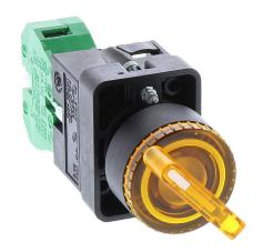
AutomationDirect selector switch, 22mm, 2-position, spring return from right, LED illuminated, (1) N.O. contact(s), plastic base, plastic bezel, Operator: yellow, knob, 30mm, round, plastic, 24 VAC/VDC, full voltage.
