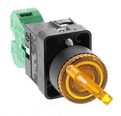
AutomationDirect selector switch, 22mm, 2-position, spring return from right, incandescent illuminated, (1) N.O. contact(s), plastic base, plastic bezel, Operator: yellow, knob, 30mm, round, plastic, 120 VAC/VDC, full voltage.
