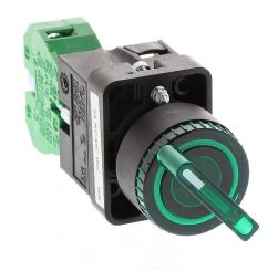
AutomationDirect selector switch, 22mm, 2-position, spring return from right, incandescent illuminated, (1) N.O. contact(s), plastic base, plastic bezel, Operator: green, knob, 30mm, round, plastic, 24 VAC/VDC, full voltage.
