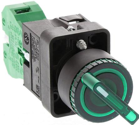
AutomationDirect selector switch, 22mm, 2-position, spring return from right, incandescent illuminated, (1) N.O. contact(s), plastic base, plastic bezel, Operator: green, knob, 30mm, round, plastic, 120 VAC/VDC, full voltage.
