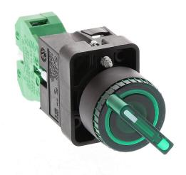
AutomationDirect selector switch, 22mm, 2-position, spring return from right, incandescent illuminated, (1) N.O. contact(s), plastic base, plastic bezel, Operator: green, knob, 30mm, round, plastic, 120 VAC/VDC, full voltage.
