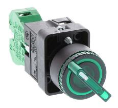
AutomationDirect selector switch, 22mm, 2-position, spring return from right, LED illuminated, (1) N.O. contact(s), plastic base, plastic bezel, Operator: green, knob, 30mm, round, plastic, 120 VAC/VDC, full voltage.
