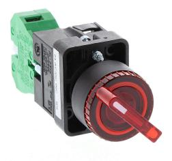
AutomationDirect selector switch, 22mm, 2-position, spring return from right, incandescent illuminated, (1) N.O. contact(s), plastic base, plastic bezel, Operator: red, knob, 30mm, round, plastic, 24 VAC/VDC, full voltage.
