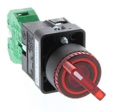
AutomationDirect selector switch, 22mm, 2-position, spring return from right, LED illuminated, (1) N.O. contact(s), plastic base, plastic bezel, Operator: red, knob, 30mm, round, plastic, 24 VAC/ VDC, full voltage.
