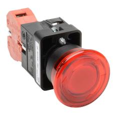
AutomationDirect pushbutton, IP65, 22mm, twist-to-release, incandescent illuminated, (1) N.C. contact(s), plastic base, plastic bezel, Operator: red, mushroom, 40mm, round, plastic, 24 VAC/VDC, full voltage.
