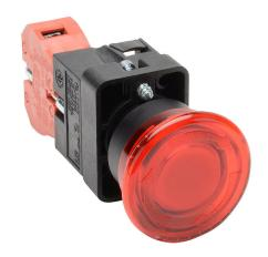
AutomationDirect pushbutton, IP65, 22mm, twist-to-release, LED illuminated, (1) N.C. contact(s), plastic base, plastic bezel, Operator: red, mushroom, 40mm, round, plastic, 24 VAC/VDC, full voltage.
