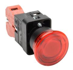
AutomationDirect pushbutton, IP65, 22mm, twist-to-release, incandescent illuminated, (1) N.C. contact(s), plastic base, plastic bezel, Operator: red, mushroom, 40mm, round, plastic, 120 VAC/VDC, full voltage.
