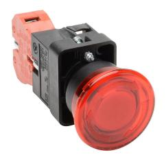
AutomationDirect pushbutton, IP65, 22mm, twist-to-release, LED illuminated, (1) N.C. contact(s), plastic base, plastic bezel, Operator: red, mushroom, 40mm, round, plastic, 120 VAC/VDC, full voltage.
