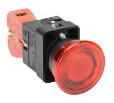
AutomationDirect pushbutton, IP65, 22mm, momentary, incandescent illuminated, (1) N.C. contact(s), plastic base, plastic bezel, Operator: red, mushroom, 40mm, round, plastic, 24 VAC/VDC, full voltage.
