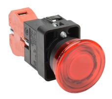
AutomationDirect pushbutton, IP65, 22mm, momentary, LED illuminated, (1) N.C. contact(s), plastic base, plastic bezel, Operator: red, mushroom, 40mm, round, plastic, 24 VAC/VDC, full voltage.
