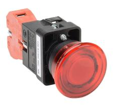
AutomationDirect pushbutton, IP65, 22mm, momentary, incandescent illuminated, (1) N.C. contact(s), plastic base, plastic bezel, Operator: red, mushroom, 40mm, round, plastic, 120 VAC/VDC, full voltage.
