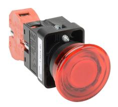
AutomationDirect pushbutton, IP65, 22mm, momentary, LED illuminated, (1) N.C. contact(s), plastic base, plastic bezel, Operator: red, mushroom, 40mm, round, plastic, 120 VAC/VDC, full voltage.
