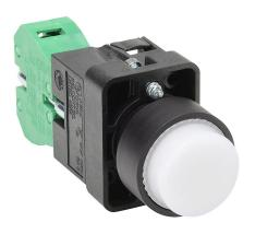
AutomationDirect pushbutton, IP65, 22mm, momentary, LED illuminated, (1) N.O. contact(s), plastic base, plastic bezel, Operator: white, extended, 30mm, round, plastic, 24 VAC/VDC, full voltage.
