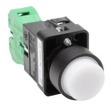
AutomationDirect pushbutton, IP65, 22mm, momentary, incandescent illuminated, (1) N.O. contact(s), plastic base, plastic bezel, Operator: white, extended, 30mm, round, plastic, 120 VAC/VDC, full voltage.
