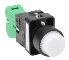
AutomationDirect pushbutton, IP65, 22mm, momentary, LED illuminated, (1) N.O. contact(s), plastic base, plastic bezel, Operator: white, extended, 30mm, round, plastic, 120 VAC/VDC, full voltage.
