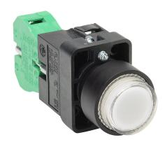
AutomationDirect pushbutton, IP65, 22mm, momentary, incandescent illuminated, (1) N.O. contact(s), plastic base, plastic bezel, Operator: clear, extended, 30mm, round, plastic, 24 VAC/VDC, full voltage.
