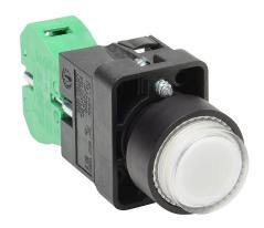
AutomationDirect pushbutton, IP65, 22mm, momentary, LED illuminated, (1) N.O. contact(s), plastic base, plastic bezel, Operator: clear, extended, 30mm, round, plastic, 24 VAC/VDC, full voltage.
