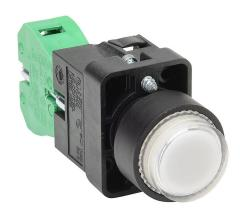
AutomationDirect pushbutton, IP65, 22mm, momentary, incandescent illuminated, (1) N.O. contact(s), plastic base, plastic bezel, Operator: clear, extended, 30mm, round, plastic, 120 VAC/VDC, full voltage.
