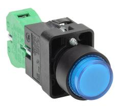
AutomationDirect pushbutton, IP65, 22mm, momentary, LED illuminated, (1) N.O. contact(s), plastic base, plastic bezel, Operator: blue, extended, 30mm, round, plastic, 120 VAC/VDC, full voltage.
