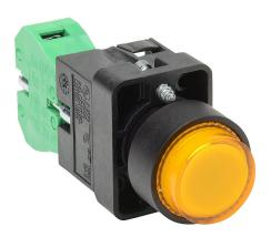
AutomationDirect pushbutton, IP65, 22mm, momentary, incandescent illuminated, (1) N.O. contact(s), plastic base, plastic bezel, Operator: yellow, extended, 30mm, round, plastic, 24 VAC/VDC, full voltage.
