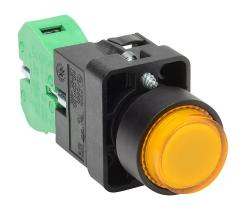
AutomationDirect pushbutton, IP65, 22mm, momentary, LED illuminated, (1) N.O. contact(s), plastic base, plastic bezel, Operator: yellow, extended, 30mm, round, plastic, 24 VAC/VDC, full voltage.
