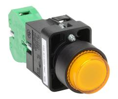
AutomationDirect pushbutton, IP65, 22mm, momentary, incandescent illuminated, (1) N.O. contact(s), plastic base, plastic bezel, Operator: yellow, extended, 30mm, round, plastic, 120 VAC/VDC, full voltage.
