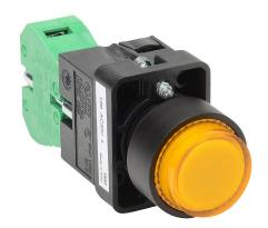
AutomationDirect pushbutton, IP65, 22mm, momentary, LED illuminated, (1) N.O. contact(s), plastic base, plastic bezel, Operator: yellow, extended, 30mm, round, plastic, 120 VAC/VDC, full voltage.
