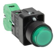
AutomationDirect pushbutton, IP65, 22mm, momentary, incandescent illuminated, (1) N.O. contact(s), plastic base, plastic bezel, Operator: green, extended, 30mm, round, plastic, 120 VAC/ VDC, full voltage.
