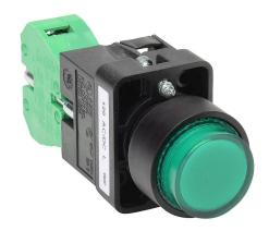
AutomationDirect pushbutton, IP65, 22mm, momentary, LED illuminated, (1) N.O. contact(s), plastic base, plastic bezel, Operator: green, extended, 30mm, round, plastic, 120 VAC/VDC, full voltage.
