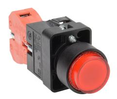
AutomationDirect pushbutton, IP65, 22mm, momentary, incandescent illuminated, (1) N.C. contact(s), plastic base, plastic bezel, Operator: red, extended, 30mm, round, plastic, 24 VAC/VDC, full voltage.
