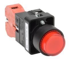
AutomationDirect pushbutton, IP65, 22mm, momentary, LED illuminated, (1) N.C. contact(s), plastic base, plastic bezel, Operator: red, extended, 30mm, round, plastic, 24 VAC/VDC, full voltage.
