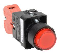
AutomationDirect pushbutton, IP65, 22mm, momentary, incandescent illuminated, (1) N.C. contact(s), plastic base, plastic bezel, Operator: red, extended, 30mm, round, plastic, 120 VAC/VDC, full voltage.
