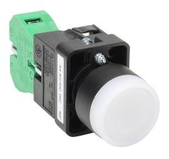
AutomationDirect pushbutton, IP65, 22mm, momentary, incandescent illuminated, (1) N.O. contact(s), plastic base, plastic bezel, plastic ring, Operator: white, flush, 30mm, round, plastic, 24 VAC/VDC, full voltage.
